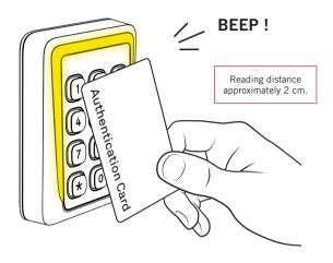
In order to set the reader in programming mode, present the valid "Authentication Card" to the reader as shown. The reader will beep and start blinking yellow to indicate that it is now in programming mode.
