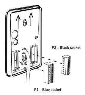
Make sure to place the terminal connectors with the fastening screws facing towards you.
