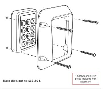
The vandalization protection is an accessory that shields the reader and helps it withstand violence by absorbing and redirecting external forces away from the reader. Can be retro-fitted to already installed readers.
