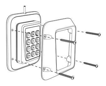
A recommended combination when external wiring is needed together with the vandalization protection. Can also be used for covering up old installation holes.
