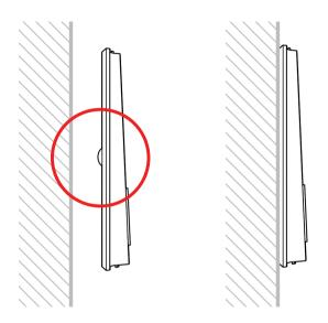
Ensure that the area behind the tamper switch bulb of the installation plate is flat, to be able to push the bulb for correct tamper alarm functionality. If it is not flat enough, you will find accessories in this manual that will assist with improving this functionality.
