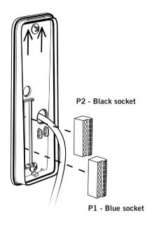
Make sure to place the terminal connectors with the fastening screws facing towards you.
