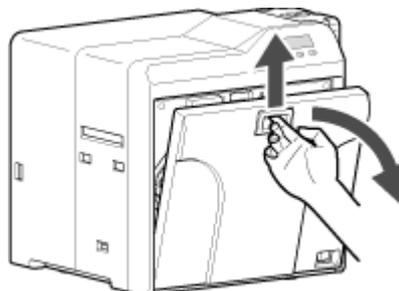
2 Press and hold down the cassette button, and pull out the retransfer film cassette (on the left) to remove the retransfer film
