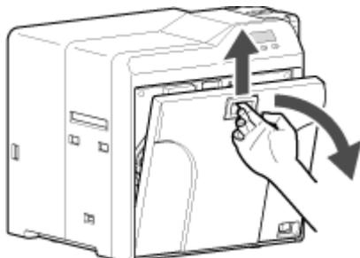
2 Press and hold down the cassette button, and remove the ink ribbon cassette (on the right) to remove the ink ribbon
