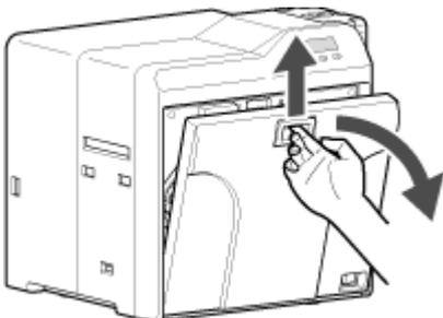
2 Press and hold down the cassette button, and remove the retransfer film cassette (on the left)
