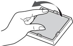
**3** Remove any dirt that is attached to the fan filter using a vacuum cleaner
