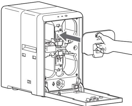
**11** Remove any slack in the laminate film
