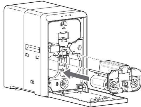
**■ If the laminate film is damaged**
