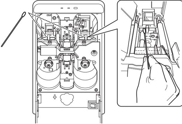
**7** Apply alcohol to a cotton swab (small), and use it to wipe the guide rail (x2) in front
