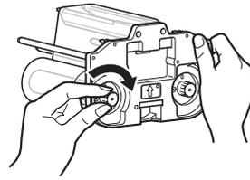
**10** Insert the film cassette all the way in along the guide rail until a “click” sound is heard, and close the laminator door
