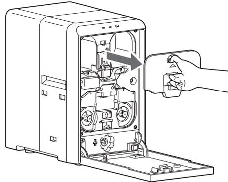
**4** Remove any slack in the laminate film
