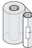
Use the fixing tape after peeling off the adhesive label of the laminate film.
