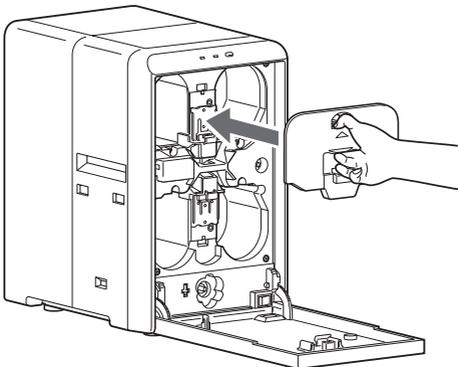
**9** Remove any slack in the laminate film
