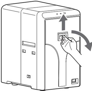
**2** Remove any slack in the laminate film
