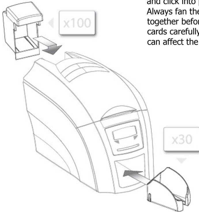
**HOPPER:** Insert the hopper into the aperture at the back of the printer and click into place.
