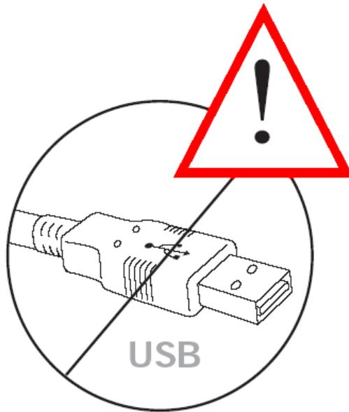
It is important to install the printer Driver first, before connecting the USB cable between your PC and ID Card Printer.
