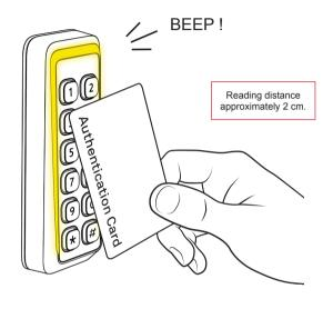
In order to set the reader in programming mode, present the valid "Authentication Card" to the reader as shown. The reader will beep and start blinking yellow to indicate that it is now in programming mode.
