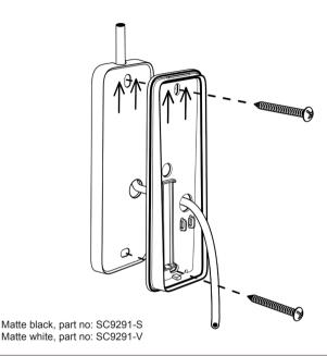
The distance plate can be used for example when installing readers in environments where the installation surface is uneven or/and external wiring at the same side as the reader.
