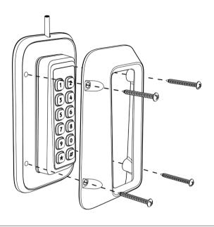
A recommended combination when external wiring is needed together with the vandalization protection. Can also be used for covering up old installation holes.
