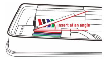
**Step 3:** Every time the RS485 communication wire is inserted into the RS232-RS485 converter, the wiring tool is inserted at a certain angle without being taken out.
