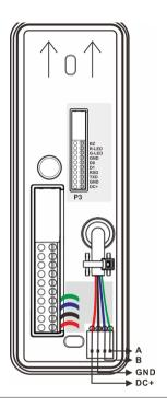
**Step 6:** Then follow the previous steps to properly connect the remaining communication wires to the converter.
