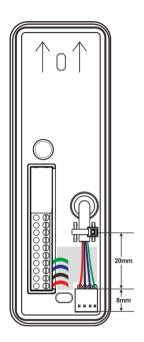
**Step 2:** The RS485 communication wires is stripped about 8 mm, then inserted into the RS485 terminal of the RS232-RS485 converter.
