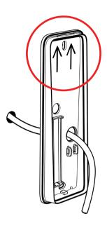
Ensure that the installation plate is fixed in the correct direction, i.e. the arrows pointing upwards.
