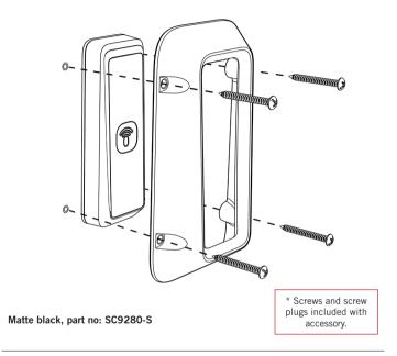
The vandalization protection is an accessory that shields the reader and helps it withstand violence by absorbing and redirecting external forces away from the reader. Can be retro-fitted to already installed readers.
