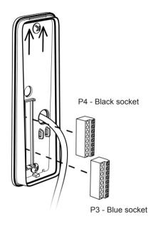
Make sure to place the terminal connectors with the fastening screws facing towards you.
