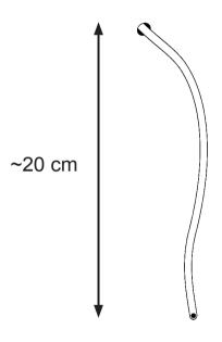
In order to facilitate installation a cable length of 20cm is recommended.
