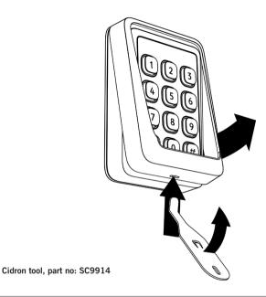
To open the reader, first remove the fixing screw and then detach the front cover from the installation plate by inserting the tip of the tool into the slot at the bottom of the front cover and move the tool upwards. This will release the front cover without damaging the front cover and/or the installation plate.
