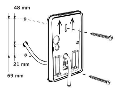
When installing directly to wall or door, use the recommended vertically aligned holes (as picture describes). If using other screws than the ones supplied with the reader, make sure to use a flat headed screw with a maximum height of 2.8 mm and a maximum diameter of 7.8 mm on the screw head.
