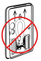
Make sure no excess connection cable is left in between the reader module and the installation plate.
