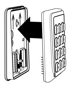
When installing the reader to the mounting plate ensure that the reader pin header contact perfectly aligns with the terminal connector block.
