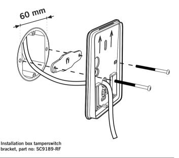
When installing reader on a installation box, use the recommended horizontally aligned holes (as picture describes). If the tamperswitch functionality should be used a installation box tamperswitch bracket must be installed between the reader and the installation box.
