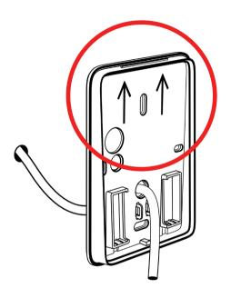
Ensure that the installation plate is fixed in the correct direction, i.e. the arrows pointing upwards.
