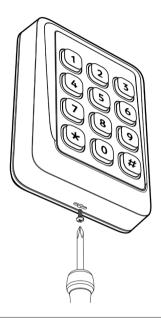
To secure the front cover to the reader use the supplied fixing screw and fix it into the installation plate through the front cover.
