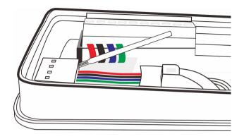
**Step 4:** The RS485 communication wire is inserted correctly into the connection hole of the RS232-RS485 converter.
