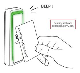
In order to set the reader in programming mode, present the valid "Authentication Card" to the reader as shown. The reader will beep and start blinking green to indicate that it is now in programming mode.
