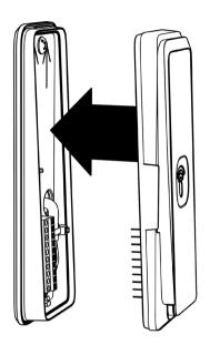
When installing the reader to the mounting plate ensure that the reader pin header contact perfectly aligns with the terminal connector block.
