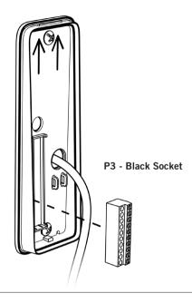
Make sure to place the terminal connector with the fastening screws facing towards you.
